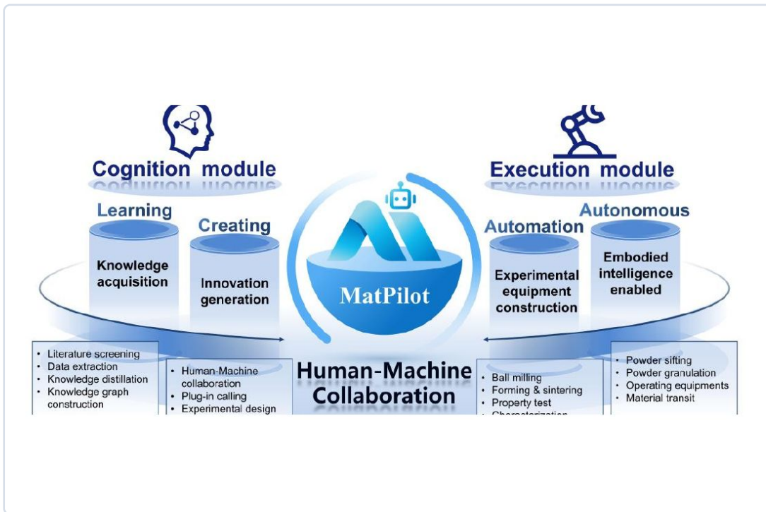
Architecture figure: MatPilot human-machine collaboration with cognition and execution modules for materials discovery.
