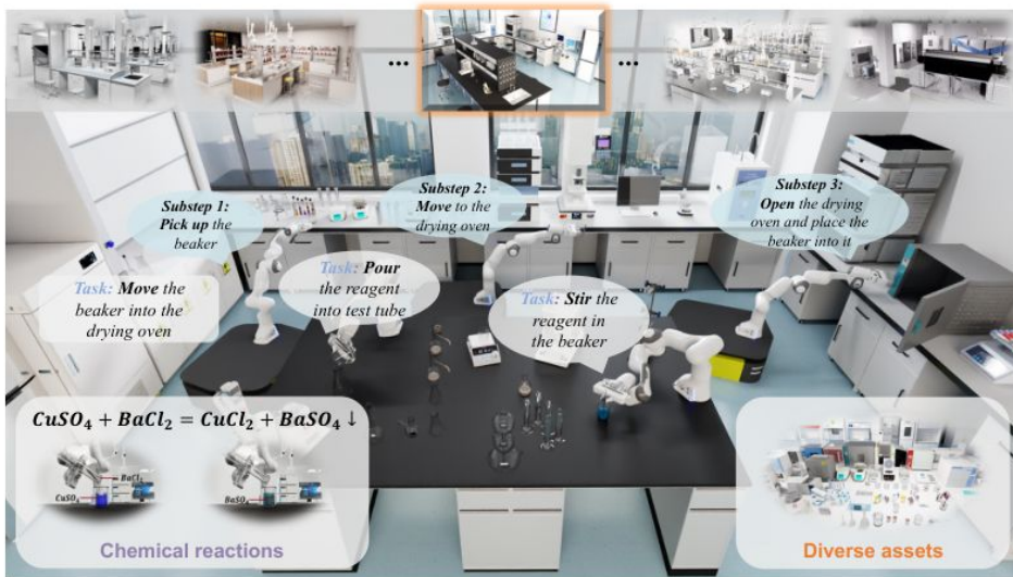
LabUtopia environment: laboratory scenes, physical/chemical interactions, manipulation/navigation tasks, and asset-rich benchmark worlds.
